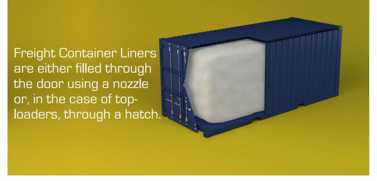
NITTEL Freight Container Liners are either filled through the door using a nozzle or, in the case of top-loaders, through a hatch. They are equipped with guide ropes, a strong corrugated cardboard door guard, metal retention bars and lateral corrugated cardboard aids for the discharging of residual product. NITTEL Freight Container Liners are suitable for all types of granulates, e.g. PE, PVC.
