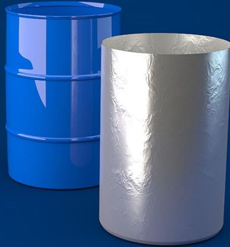
NITTEL Barrier Foil Round Bottom Liners are manufactured by welding a circular disc to one end of an open ended tube of material. The weld then forms a liquid tight seal. This technology provides a high level of tear resistance. The accurate fit of the liner reduces the formation of creases and air pockets, which is often a problem with ordinary flat bags.
